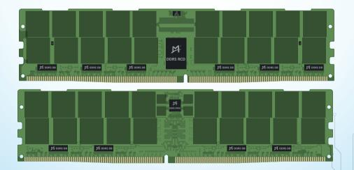
Note: The image above uses DDR5 LRDIMM as an example to showcase the application of our DDR5 memory interface chips. To represent a DDR5 MRDIMM / MCRDIMM configuration, simply replace the RCD and DB with MRCD and MDB respectively.
